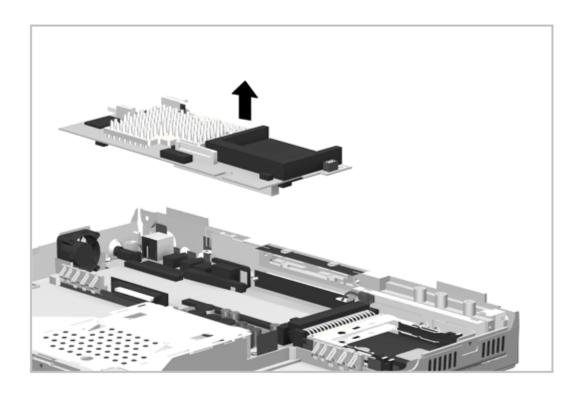
Figure 5-51. Removing the Processor Board
